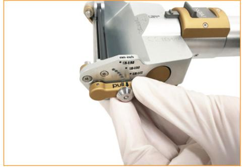
Figure 5. Adjust cutting thickness
